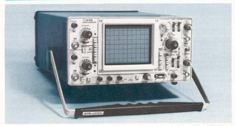
475 pictured above is identical in appearance to the 465 (not shown) except the 465 deletes the 0.01 and 0.02 μs TIME/DIV and 2 mV VOLTS/DIV switch positions.
